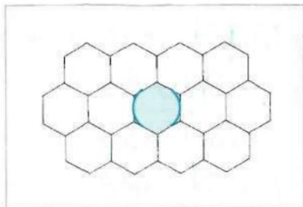
The camera's standard metering mode is AF-Integrated, 14-Segment, Honeycomb-Pattern Metering, which will provide the correct exposure in almost all situations. Spot metering can also be manually selected, in which case, the center segment in the honeycomb pattern is used exclusively to measure the subject's brightness.
