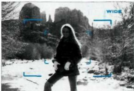
This feature enables you to see the area immediately outside of the film frame up until the moment that you press the shutter-release button.
