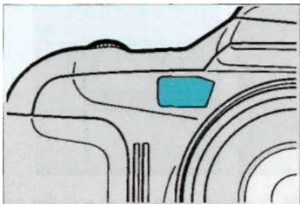
In low-light or when subject contrast is too low to be read by the autofocus sensors, the AF illuminator will activate. It projects a pattern of lines onto your subject which the AF sensors can then detect.
