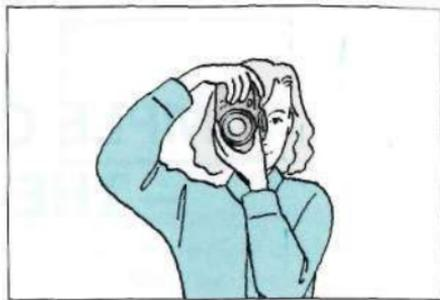
Hold the grip firmly in your right hand and use your left hand to support the camera or lens. Keep your elbows securely against your sides when shooting both horizontal and vertically pictures. Press the shutter-release button gently in a single, steady motion—never with a quick jab. Always keep the camera strap around your neck or wound around one wrist.
