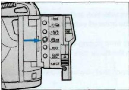
To begin rewind at any time, open the card door and press the rewind button.
