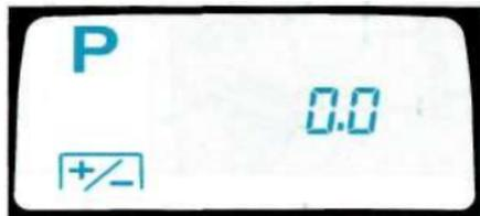
This function enables you to bias the camera's exposure calculation up to +/- 4 stops.
