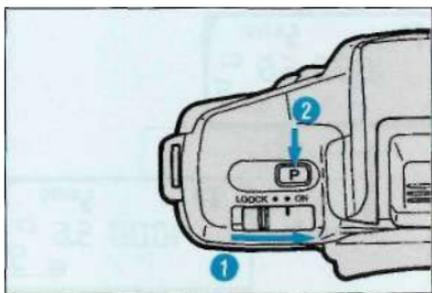
1. Slide the main switch to ON and press the program-reset button to set full-automatic operation.
