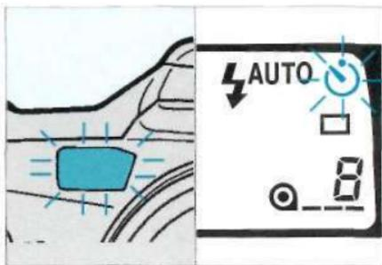
The electronic self-timer will delay release of the shutter about 10 sec. after you press the shutter-release button.
