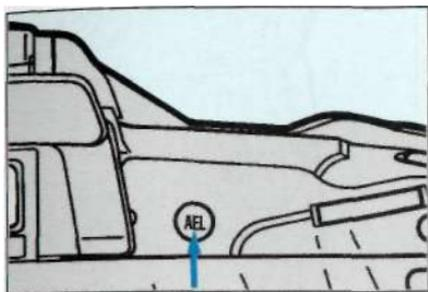
3. Continue to hold the AE lock button and press the shutter-release button down completely.
