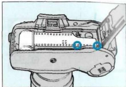
1. Open the back cover by sliding the back-cover release downward.
