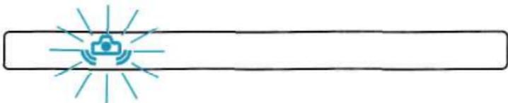
When your subject or scene is too dark to allow a clear hand-held photograph, the camera-shake warning will blink in the viewfinder data panel. The built-in flash will pop-up automatically, if it is required, when you press the shutter-release button partway down and will fire when you take the picture. You should also consider using a tripod.
