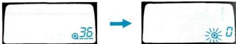
After you have exposed the last frame, the camera will automatically rewind the film. With a fresh battery, it takes about 9 sec. to rewind a 36-exposure roll, or 6 sec. for a 24-exposure roll. When the film has been completely rewound, the motor will stop and the film-cartridge symbol in the body data panel will blink to indicate that it is safe to open the camera back.
