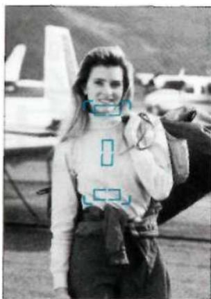
The autofocus system uses expert programming and fuzzy logic to determine which of the AF sensors is detecting your main subject. The camera's ultra-wide AF area has four sensors—two vertical and two horizontal. When you hold the camera horizontally, all four sensors are active; when you hold the camera vertically, the top horizontal sensor shuts off and the AF area changes to its vertical mode.
