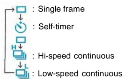
3. To return to single-frame advance, press the self-timer/drive-mode button until it appears in the data panel.
