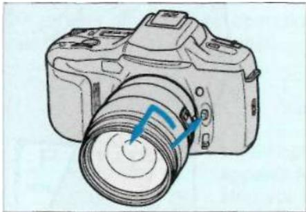
1. While pressing the lens release, turn the lens counterclockwise until it stops. Lift the lens out of the mount.
